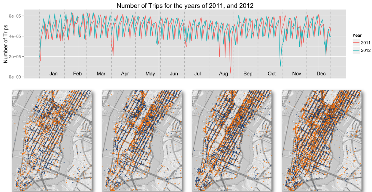
Fig. 2. Taxis as sensors of city life. The plot on the top shows how the number of trips varies over 2011 and 2012. While some patterns are regular and appear on both years, some anomalies are clear, e.g., the drops in August 2011 (Hurricane Irene) and in October 2012 (Hurricane Sandy). In the bottom, we show pickups (blue) and dropoffs (orange) in Manhattan on May 1st from 7am to 11am. Notice that from 8-10am, there are virtually no trips along 6th Avenue, indicating the traffic was blocked.
