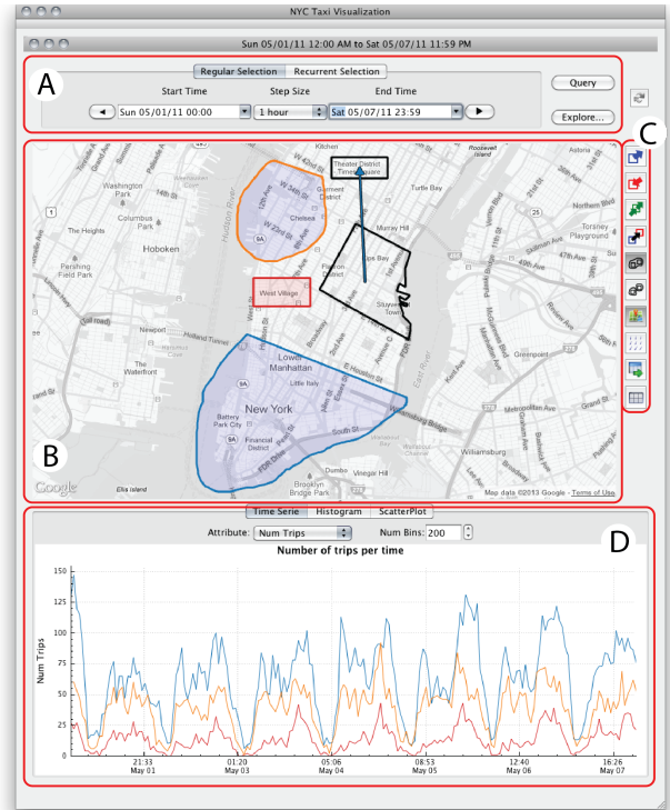
Fig. 4. TaxiVis user interface components. (A) Time selection widget, (B) Map, (C) Tool bar, and (D) Data summary. We can also see an example of three distinct queries specified by colors. The orange query (orange border polygon) represents an atomic query with a spatial single region start constraint. The red query (red border polygon) represents an atomic query with a spatial single region end constraint. The blue query is a complex query which is the union of two atomic queries: the polygon with blue border (atomic single region start constraint) and a directional query (blue arrow).
