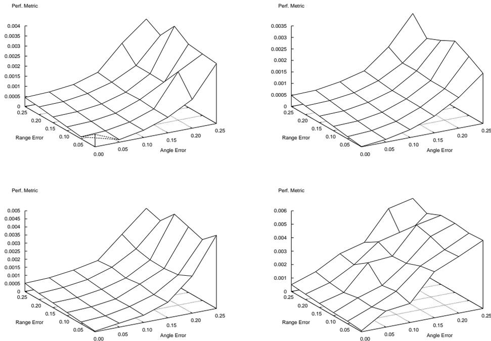
**Fig. 10.** Using the GER metric: Error tolerance for MSDR across triangle-shape, square-shape, star-shape and U-shape graphs with sizes 500. There were five trials per for each experiments, using graphs with density 16 and varying the range errors and the angular errors.
