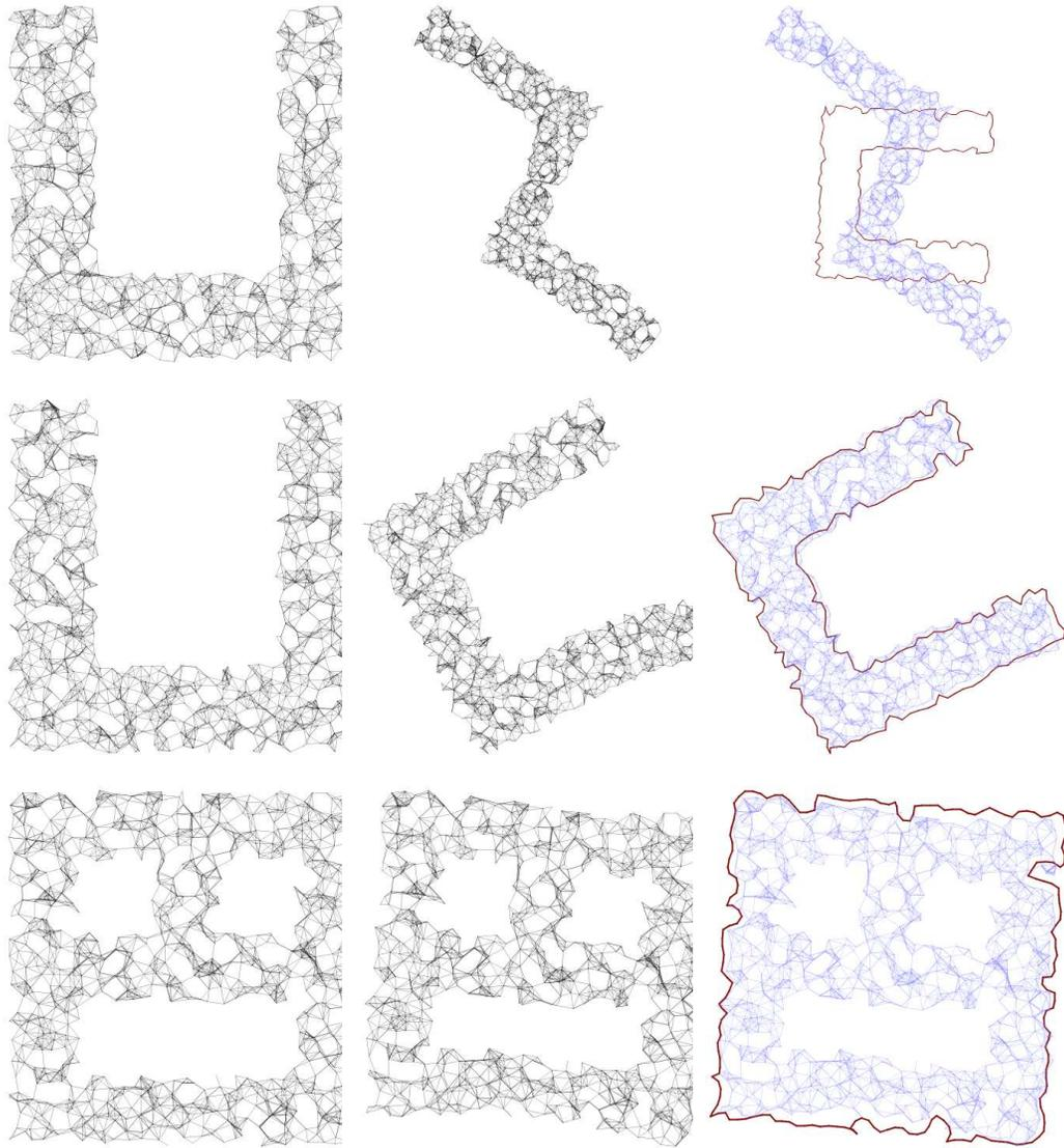
**Fig. 8.** Some typical input/output pairs illustrating input/output/boundary for MSKKR (top) and MSDR (middle and bottom). The underlying graphs have 1000 vertices, density 8, range error of 10% and angle error also 10%.
