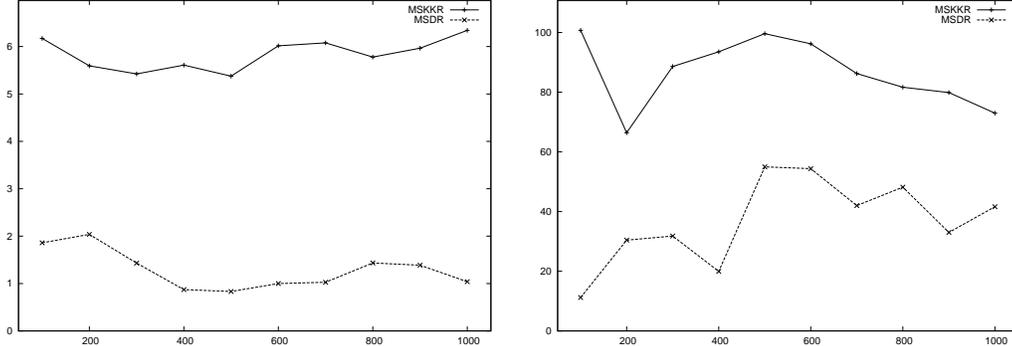
**Fig. 7.** Comparison between MSKKR and MSDR measured by the BAR metrics across square-shape and U-shape graphs with sizes 50 to 1000. There were five trials per shape, using graphs with density 8 and 10% range errors and 10% angular error.
