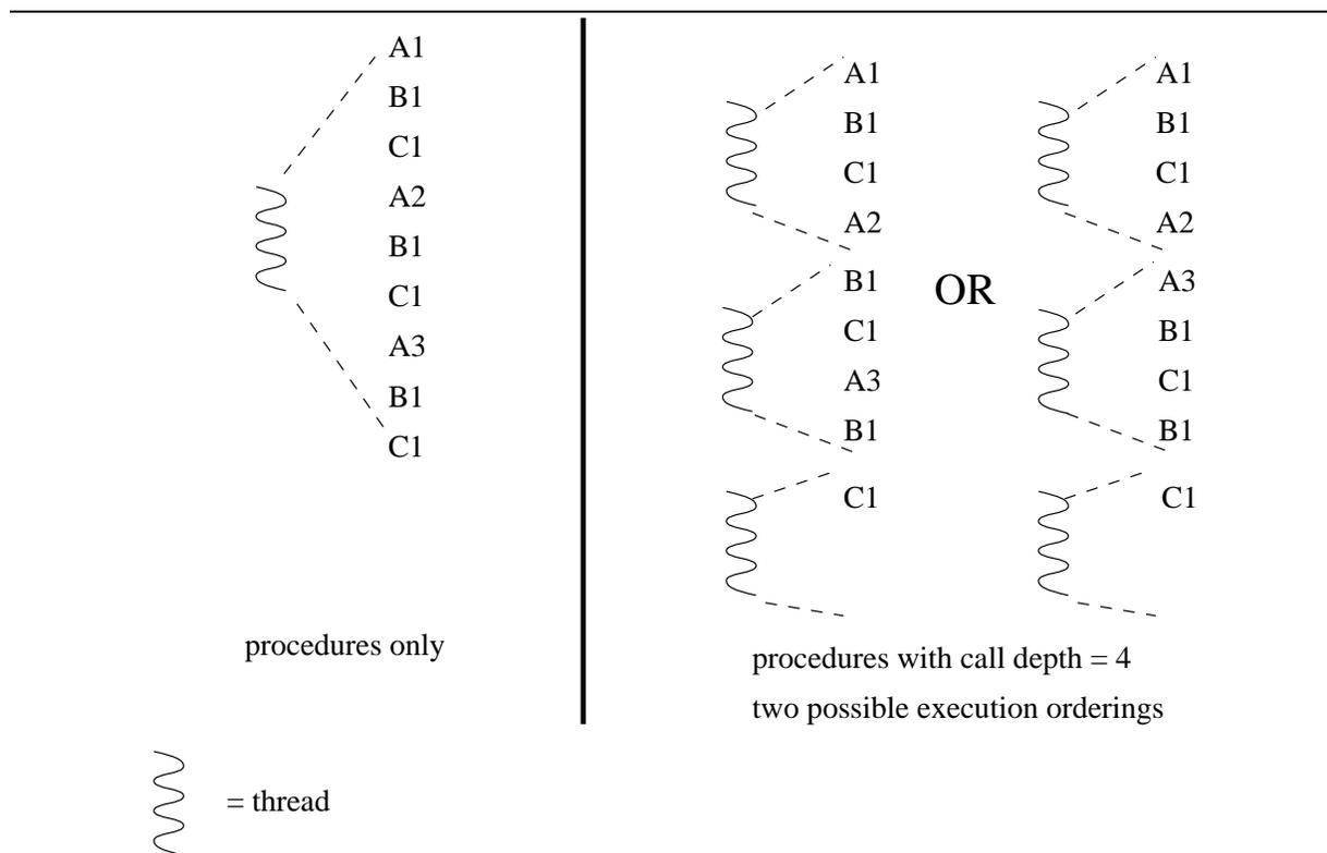
Figure 5: Possible event handler executions with and without call depth bounding.
