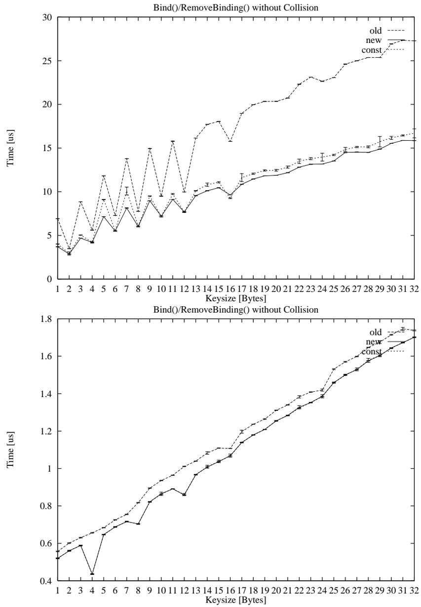
Comparing the following graphs with the ones above, it becomes clear that collisions during insertion/removal have only a minor impact on performance.
